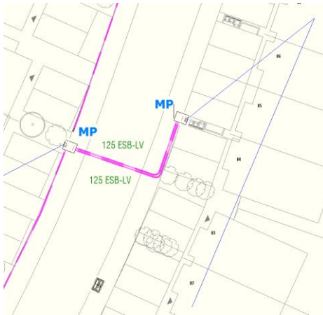
Figure 16-4 Sample of ESB mini-pillar and in ground ducting including run outs to Dwellings
