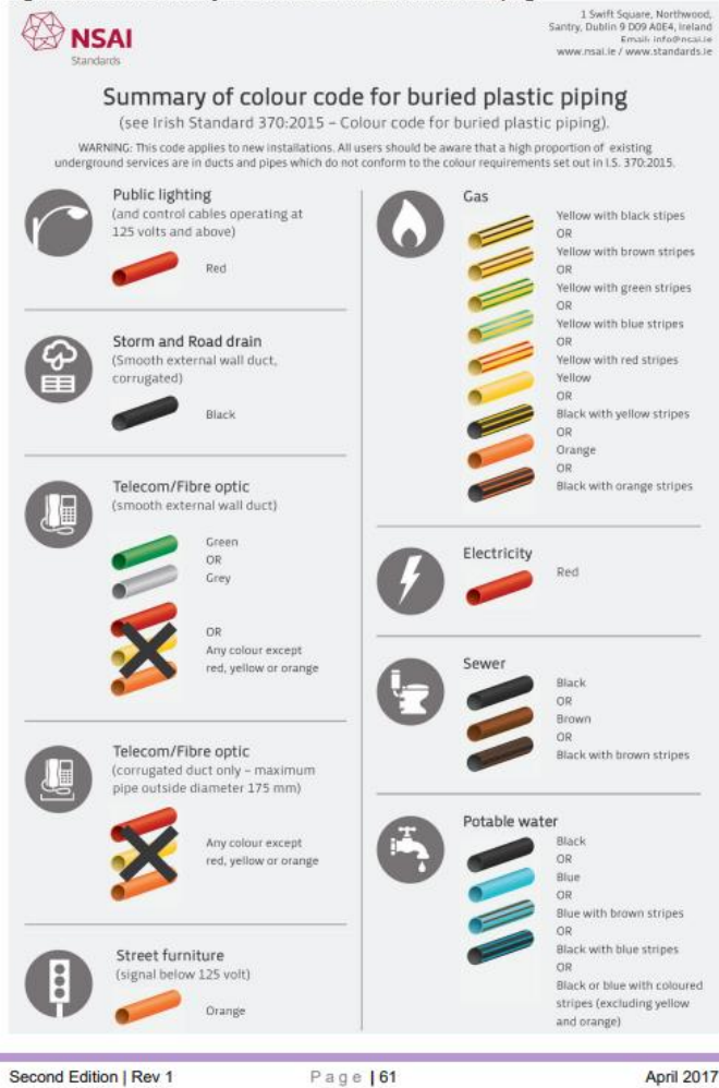
Figure 6.2.1 NSAI Summary of Colour Code for Buried Plastic Piping
